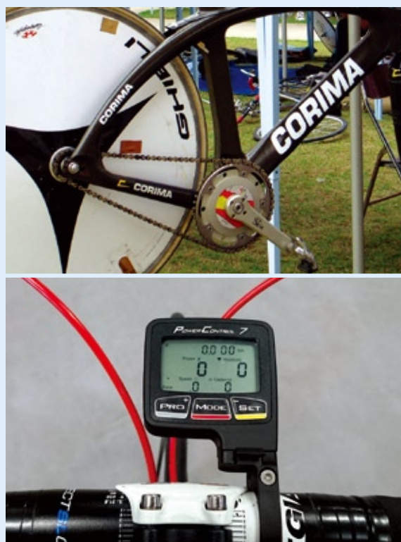
Figure 3.2 Powermeter (left) and powercontrol (right) of SRM system
